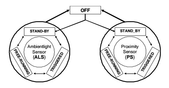
If  $V_{\rm DD}$  exceeds the threshold-voltage, the sensor will switch from OFF to STAND-BY mode. As shown in the transition diagram above it is possible to switch between all modes without any restriction. The transition time between modes ( $t_{\rm trans}$ ) is < 10ms. The delay time between STAND-BY and start of measurement is max. 10ms for the Ambient Light Sensor.
